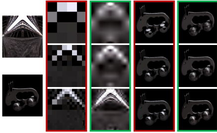
Figure 1: Iterative refinement of illumination by adding detail coefficients based on a splitting criterium. Reconstructions for both Haar (red) and the smoother Coiflet (green) wavelet bases are shown. Haar has a tendency to introduce disturbing high frequencies around edges.
